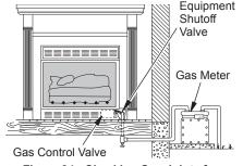
Figure 24 - Checking Gas Joints for Natural Gas
